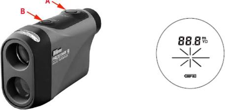
To take a measurement press the Power button **A** and the LCD illuminates, align the reticle on the target and press and hold the Power button again until the display appears as it does in the picture, right side above. To obtain the best results try to select bright colored targets with large, shiny, highly reflective surfaces.
