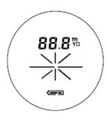
To take a measurement press the Power button **A** and the LCD illuminates, align the reticle on the target and press and hold the Power button again until the display appears as it does in the picture, right side above. To obtain the best results try to select bright colored targets with large, shiny, highly reflective surfaces.
